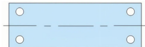
Figure 2: Bearing Layout Example for Simply Supported Box Girder
